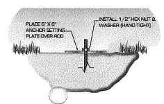
5 With the deep wall socket and 3/8" drill, tighten down on the hex nut. As the threaded rod is drawn up the anchor will set itself to the anchored position. There must be 4" to 6" of threaded rod above ground when the anchor is set. Remove the nut and anchor setting plate and keep for the next installation.
