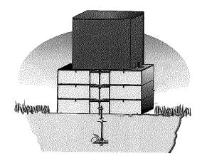
10 Attach the clips to the MESA first - use a 3/8" bit to drill through the hole in the clip and though the top of the MESA. With the clip placed over the hole, push an AVK fastener through the hole in the clip and through the hole in the MESA. The fastener sits on top of the clip - not under it.
