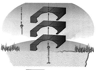
Using care, place the densing unit on top of the MESA. <u>Do not drop</u>! The raise dreas on the top surface of the MESA will indicate the best position for the unit and fastening clips. Determine the correct condenser position and all 4 clip locations before you drill.
