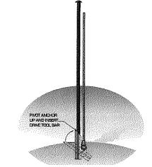
3 Hold the threaded rod and the drive tool together in one hand and use the sledge to hammer the drive tool, threaded rod and anchor into the ground.
