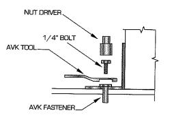
11 Place the fastener tool over the fastener flange and thread a 1/4" x 20 x 1-1/4" S.S. bolt through the hole in the tool and into the fastener a few turns to get it started. Use a variable speed drill with a 7/16" nut driver - apply some downward pressure and turn the bolt until it pulls the fastener tight. The fastener tool helps to keep the fastener from spinning out. <u>Remove the bolt to release the fastener tool</u>.
